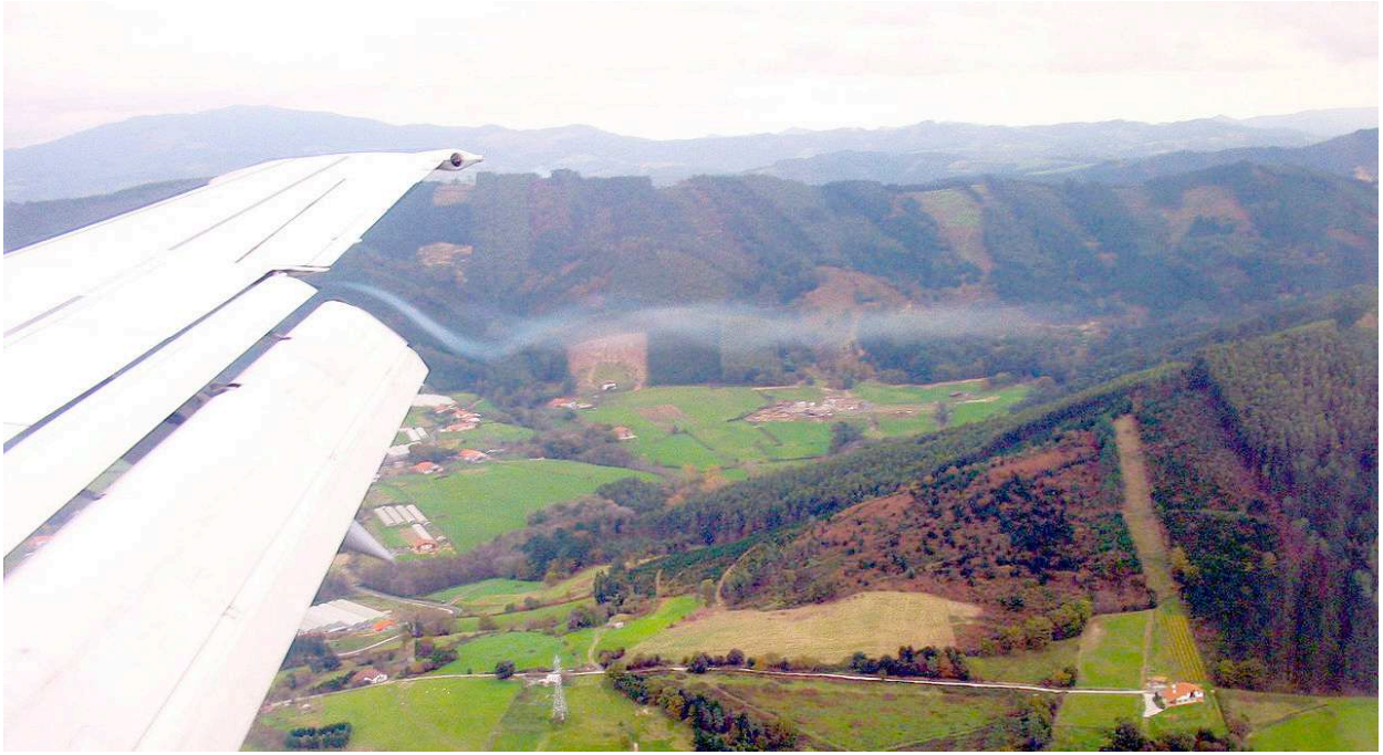
Figure 10.5: Vortex caused by flap illustrating the creation of vortices in locations where lift distribution changes rapidly. (November 28, 2006. Author: Miguel Andrade. Public domain image).
