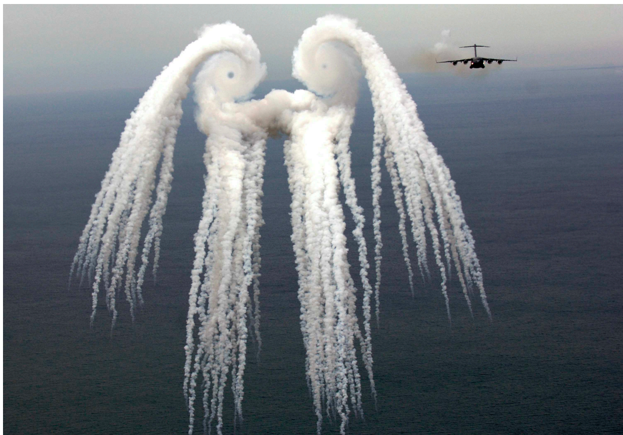
Figure 10.4: Wingtip vortices on a C-17 Globemaster III highlighted by smoke from flares. (U.S. Air Force. Author: Tech. Sergeant Russell E. Cooley IV. May 16, 2006. Public domain image).
