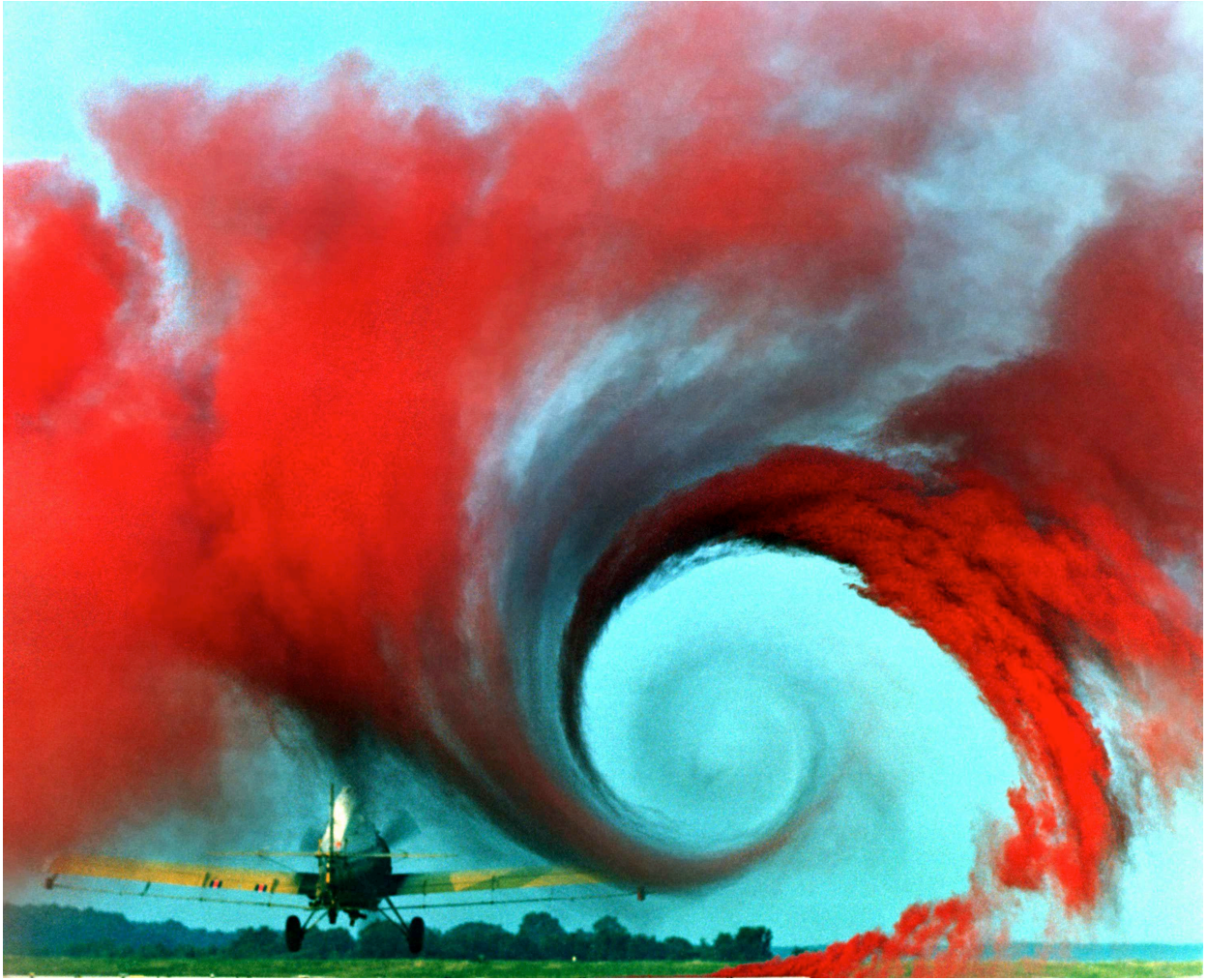
Figure 10.3: Wing tip vortex of an agricultural plane highlighted by a colored smoke rising from the ground. (NASA Langley Research Center. Photo ID: EL-1996-00130. Public domain image).
